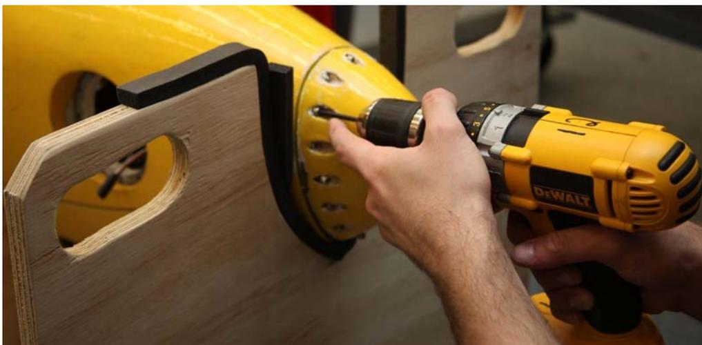
Figure 73: Removing Nosecone Assembly
