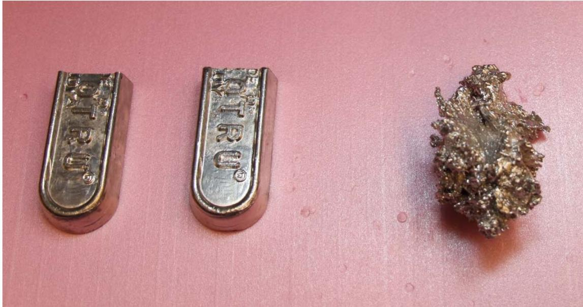
**Figure 9: Bismuth/Tin Alloy for Ballast**
