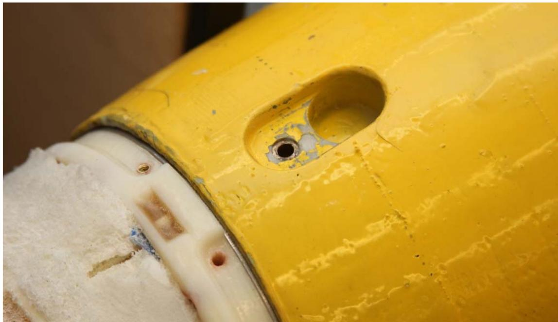
Figure 12: Dorsal Fin On/Off Switch in Hull
