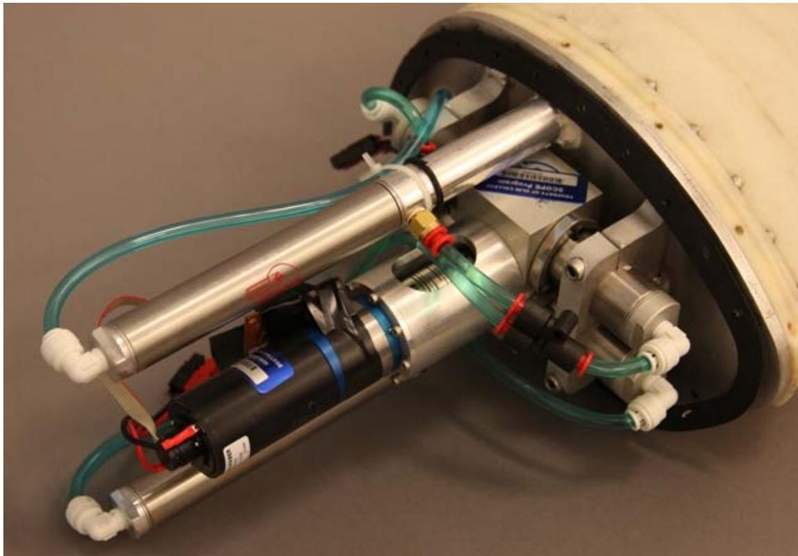
**Figure 49: Hydraulic Transmission**
