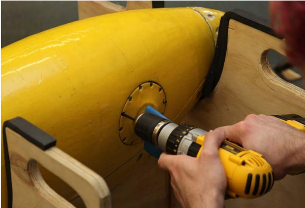
Figure 72: Removing Pectoral Fin Assembly I
