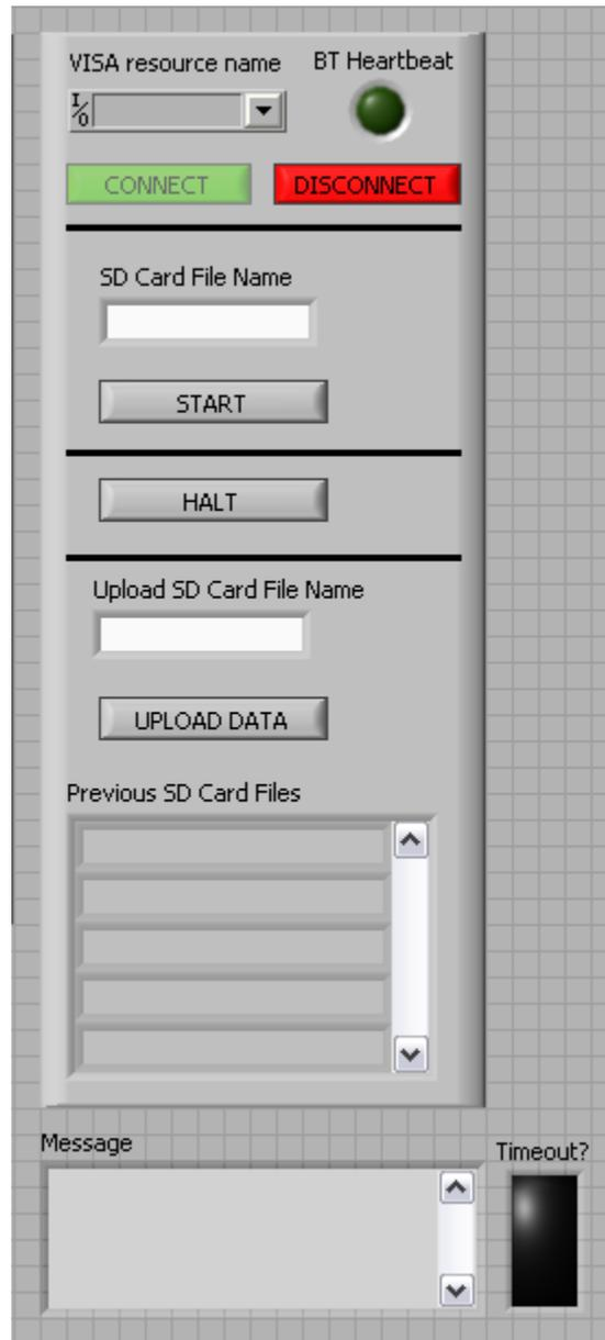
**Figure 34: Bluetooth from Laptop: Front Panel**
