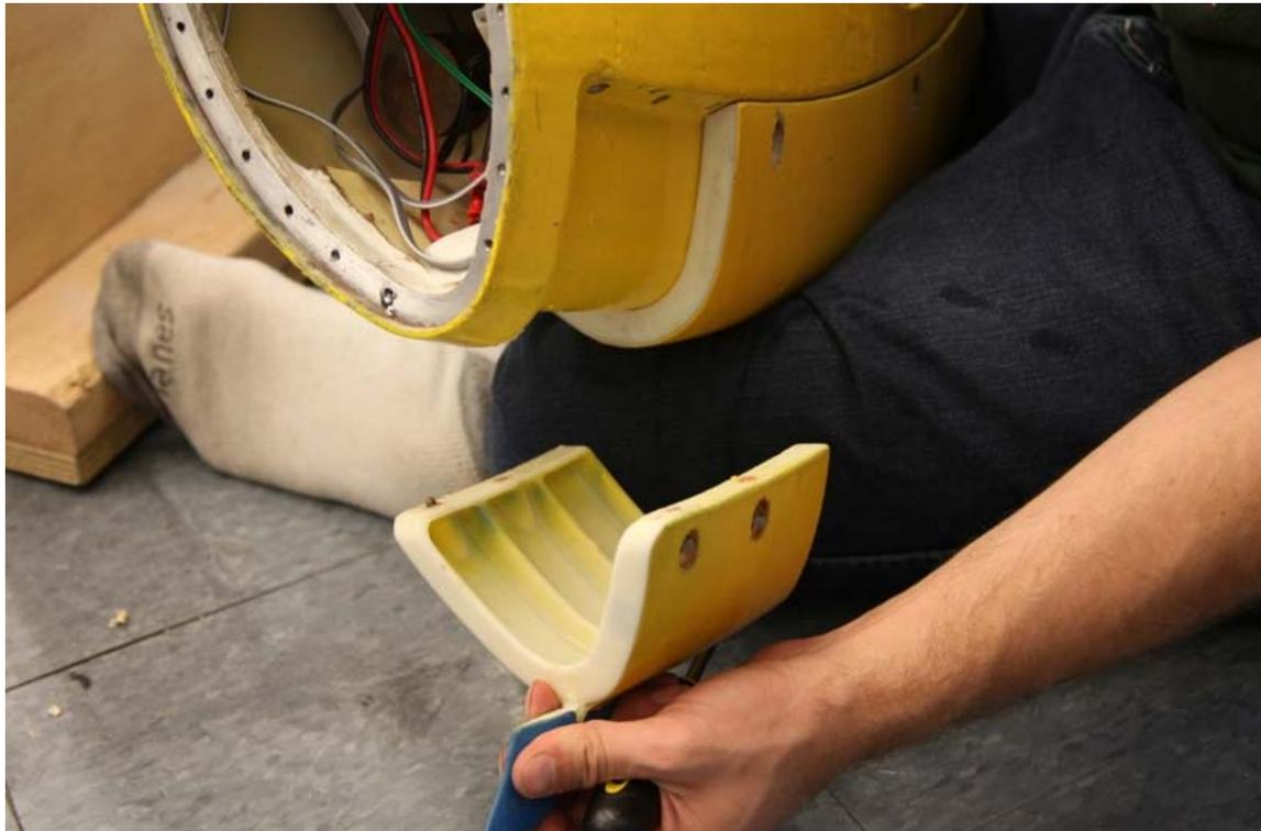
**Figure 61: Installing Front Ballast Compartment**
