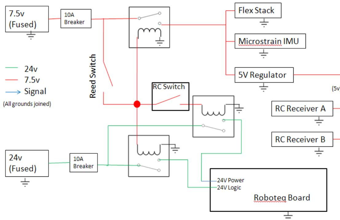
Figure 25: Power Distribution Diagram
