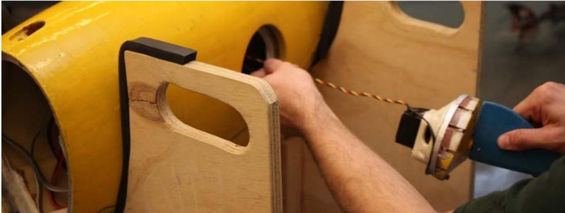
**Figure 74: Removing Pectoral Fin Assembly II**
