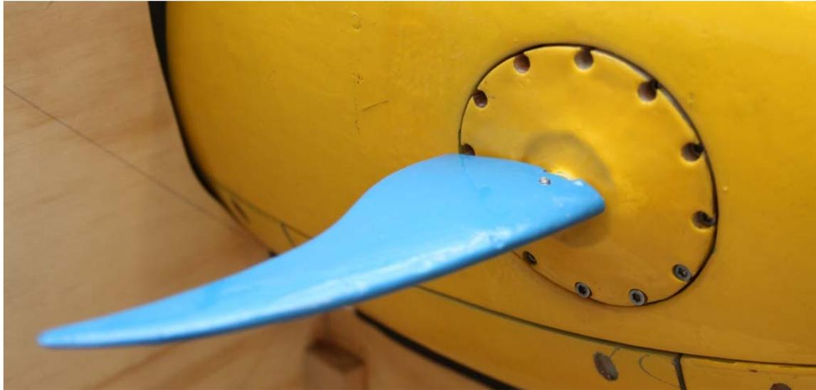
Figure 22: New Pectoral Fin Joint Installed in Hull
