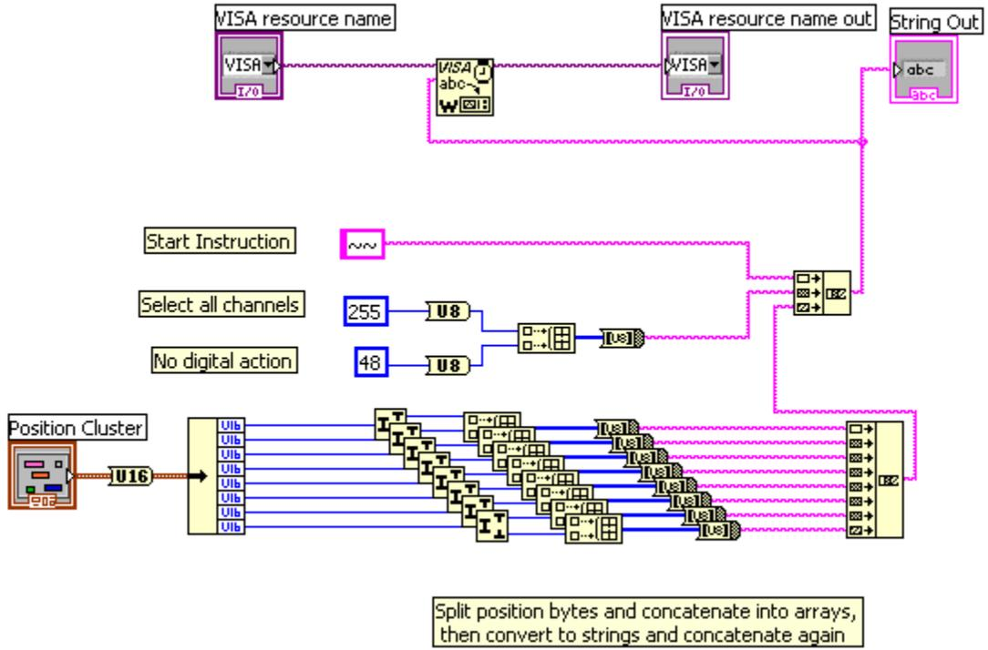
Figure 82: RC Control Driver.vi Block Diagram
