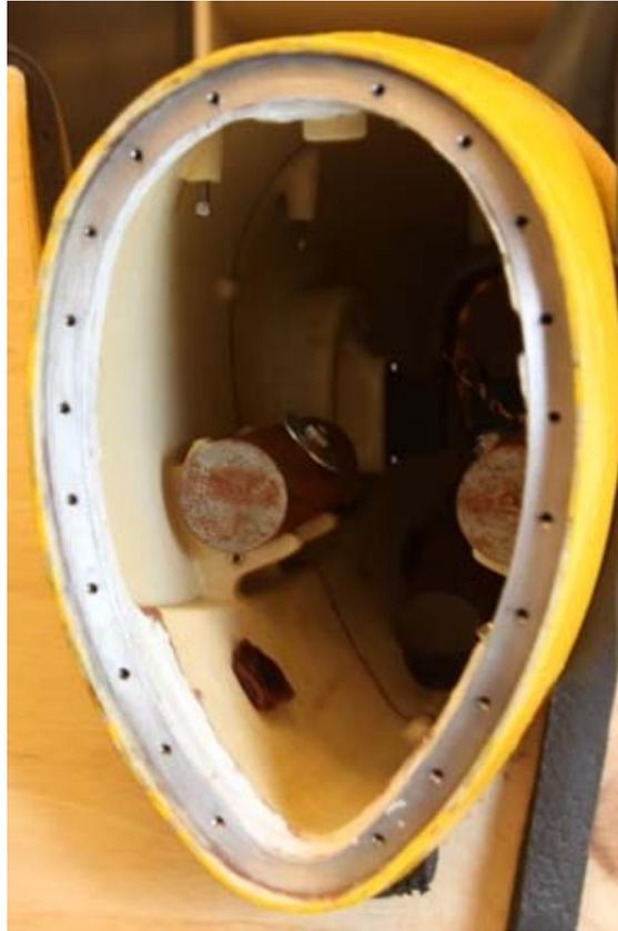
Figure 5: Main Hull Seal
