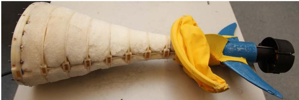
Figure 14: Foam Sections in Final Tail
