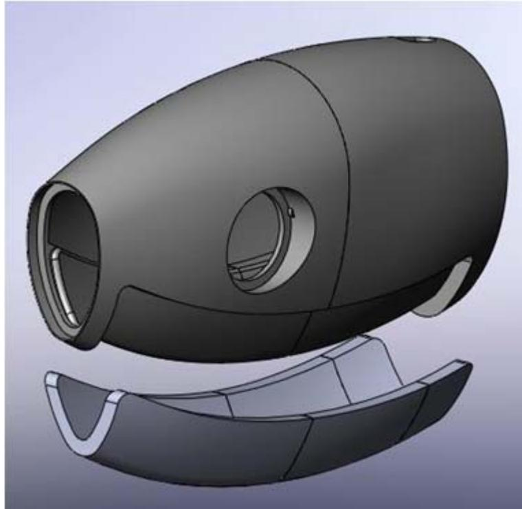
**Figure 10: New External Ballast System Design**
