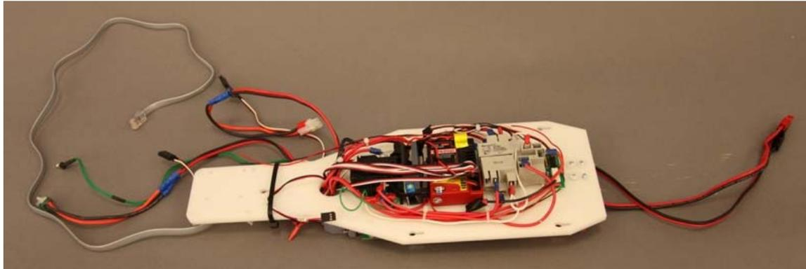
**Figure 53: Electronics Board Top View**
