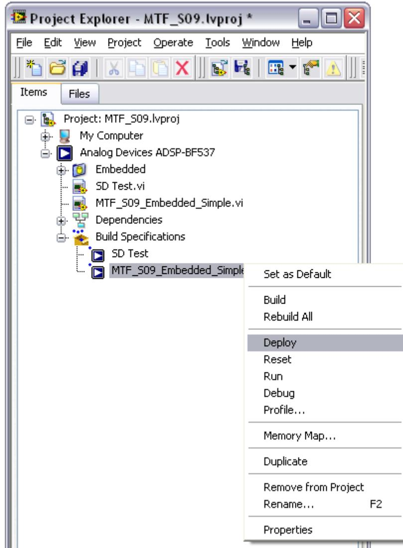
Figure 32: Deploying Embedded Code
