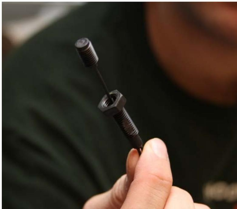
**Figure 75: Damaged Reed Switch**
