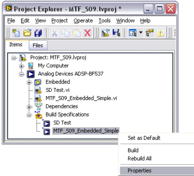
Figure 37: Accessing Build Properties
