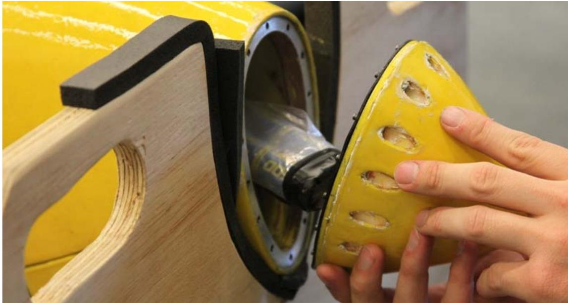
Figure 62: Installing Nosecone Section I
