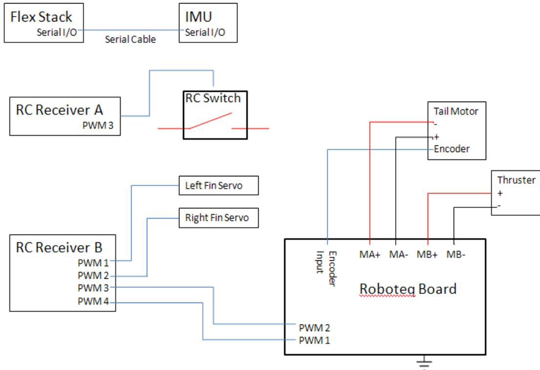
Figure 26: Motor Connections Diagram
