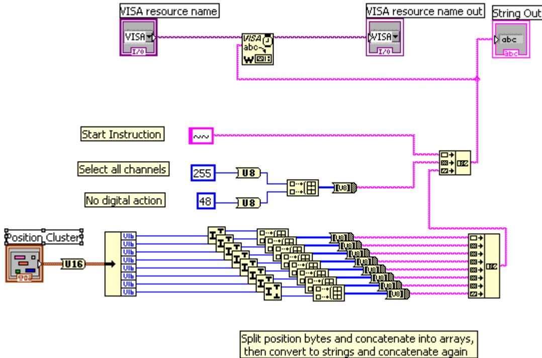
Figure 31: RC Control Driver Block Diagram
