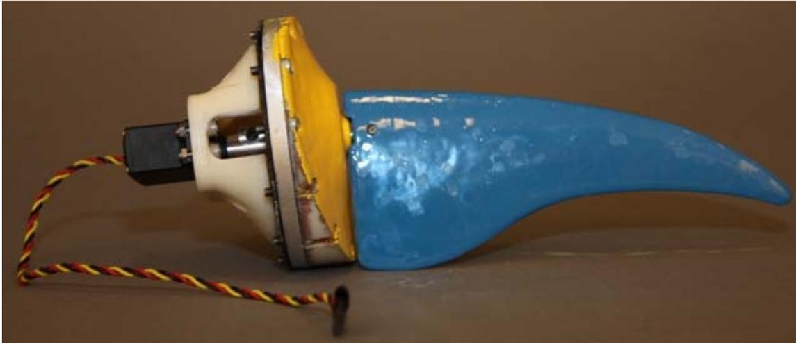
**Figure 46: Pectoral Fin Assembly Side View**
