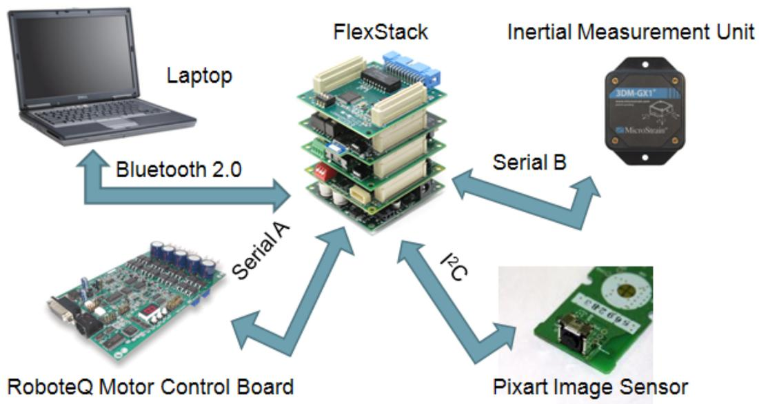
Figure 39: Suggested Sensor Suite for Autonomous Swimming
