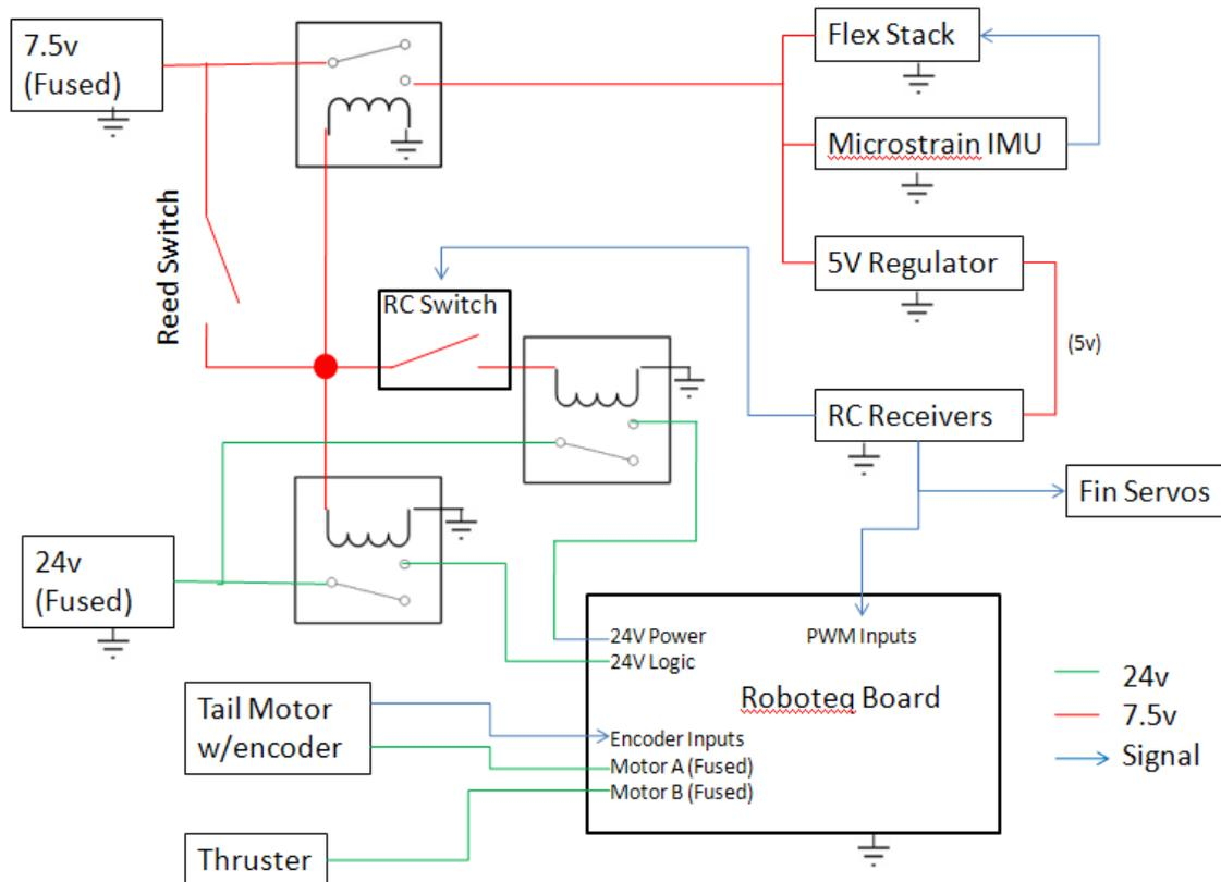
Figure 24: Electronics Wiring Diagram
