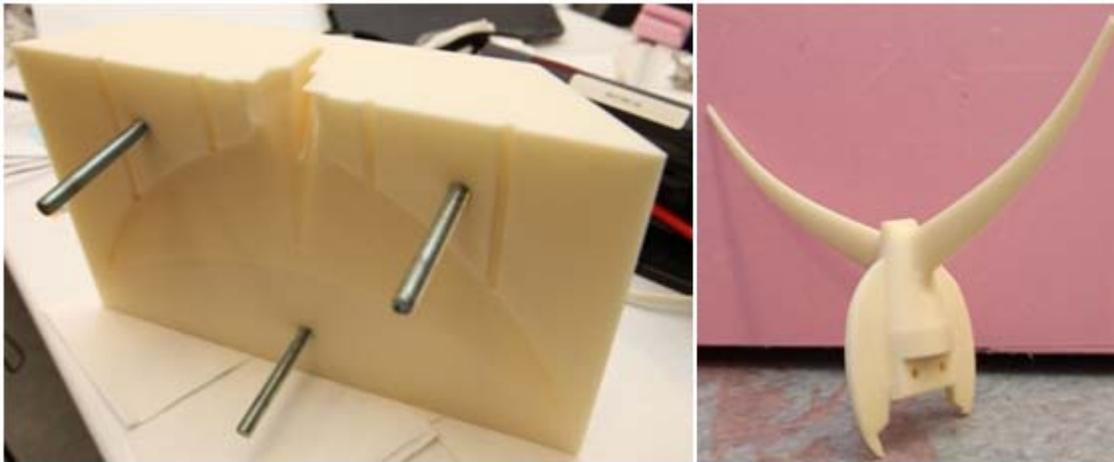
**Figure 18: Flexible Caudal Fin Mold and Spine**
