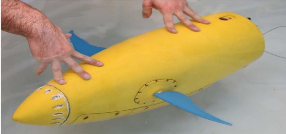
**Figure 41: Testing New Static Hull Seals**
