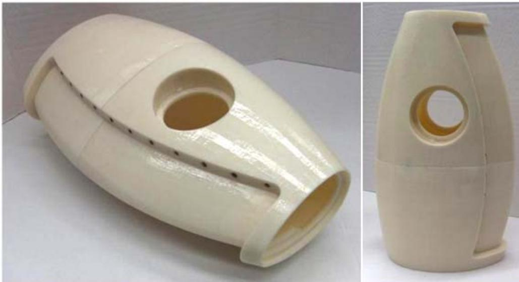
Figure 7: New Hull RP Parts
