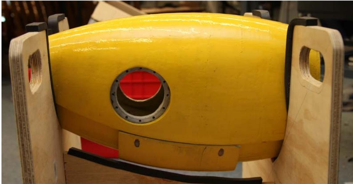
Figure 59: Hull with Middle Ballast Section Attached
