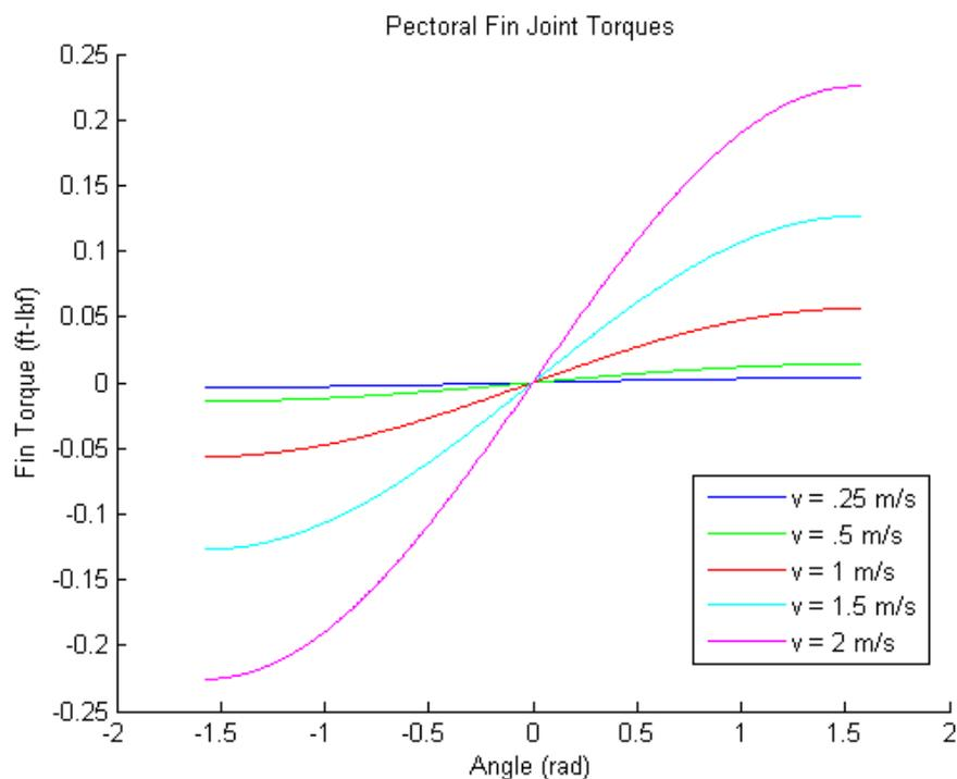
Figure 40: Angle vs Torque for Pectoral Fins
