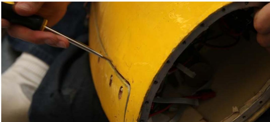
Figure 60: Removing Rear Ballast Compartment
