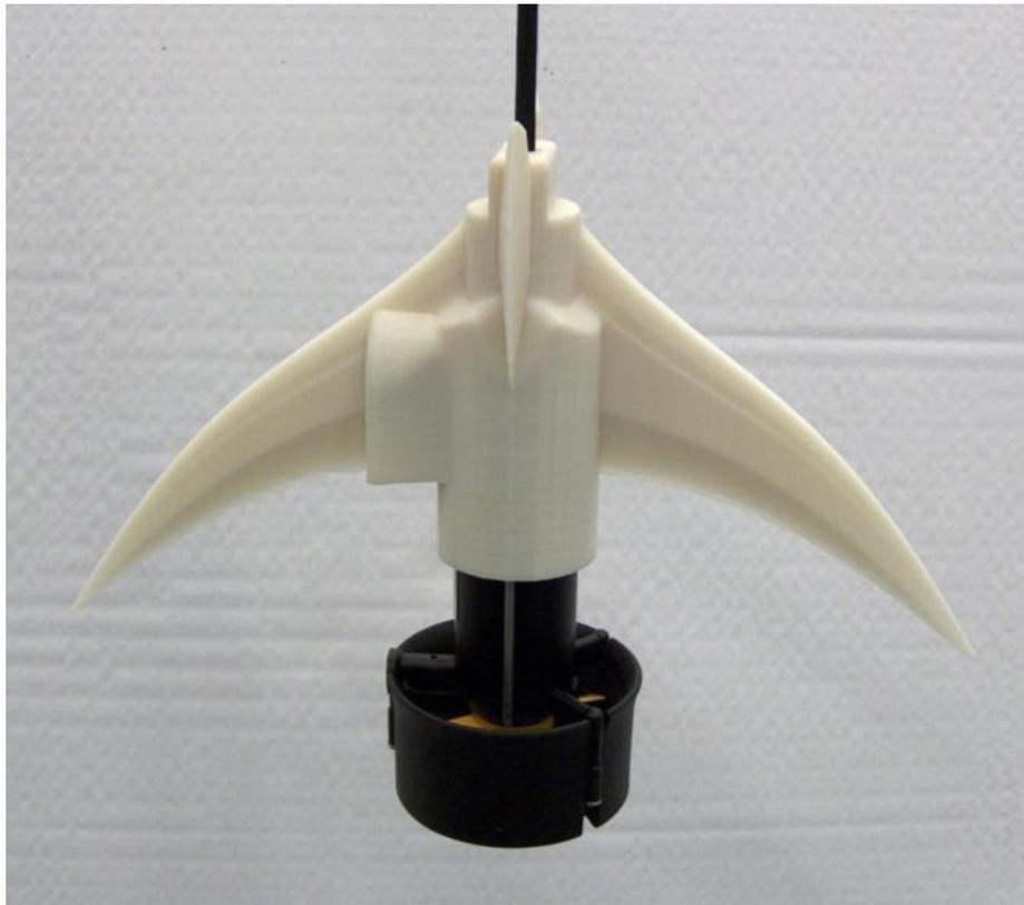
**Figure 16: New Caudal Fin With Built-In Finlets**
